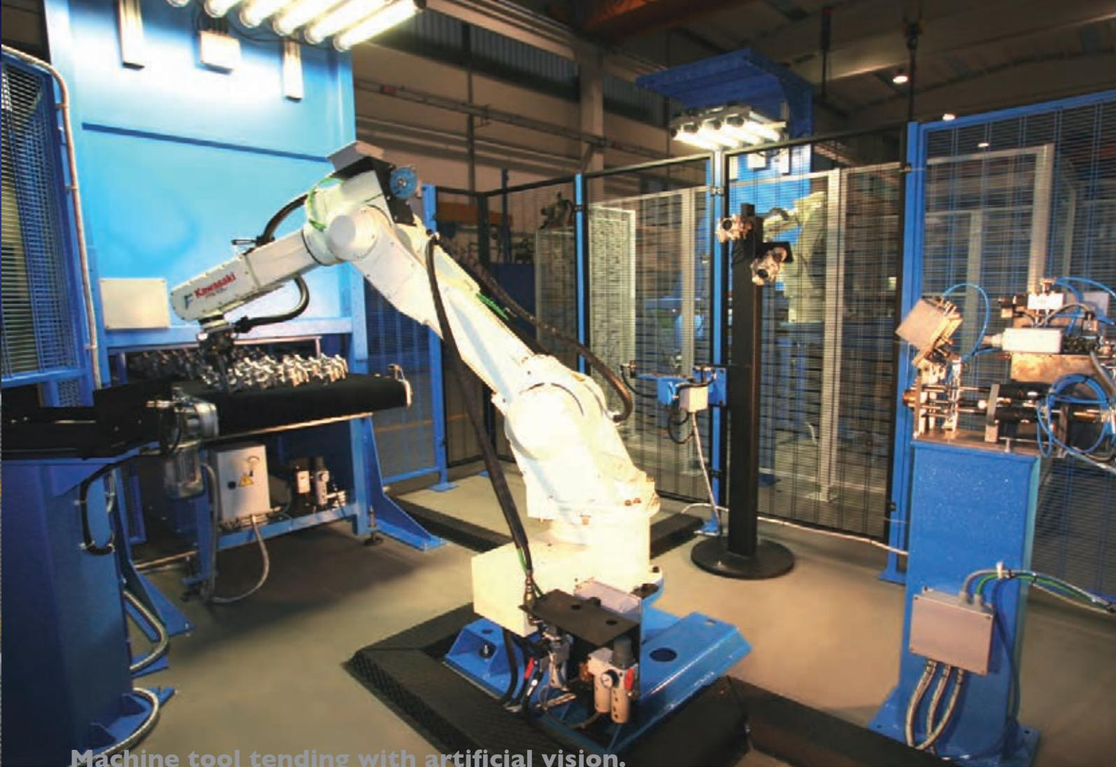
**Machine tool tending with artificial vision.**
